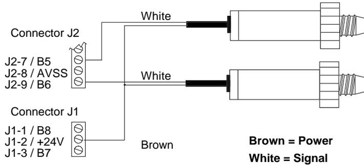
Connect the transducers directly to the interface
