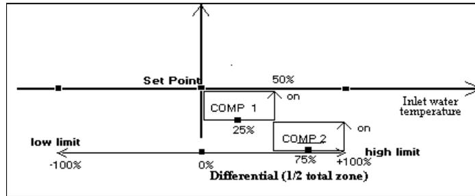
**Note:** the example above refers to cooling applications (Summer mode). For heating applications (Winter mode), the steps will be positioned specularly with respect to the set-point.
