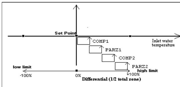
**Note:** the example above refers to cooling applications (Summer mode). For heating applications (Winter mode), the steps will be positioned specularly with respect to the set-point.
