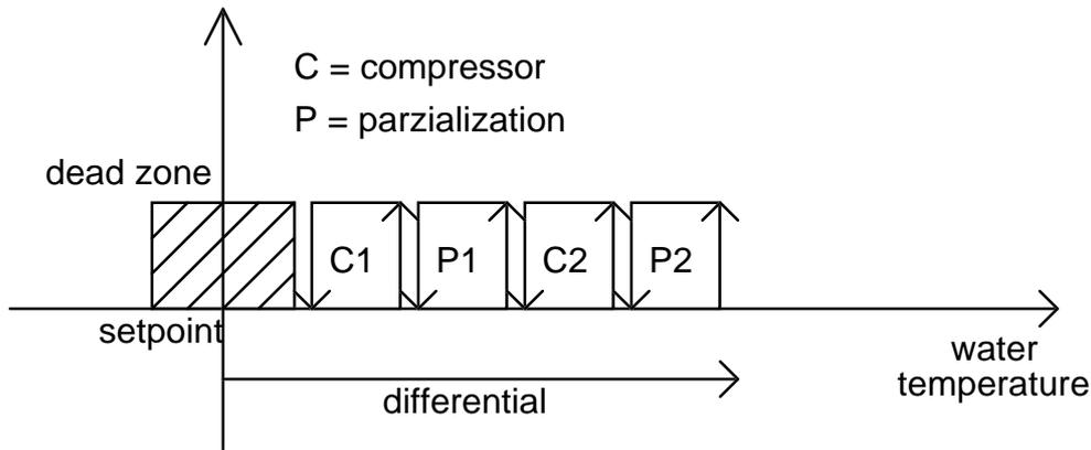
**Note: the range of the dead zone must be inferior to the selected differential otherwise the connected devices will not activate.**
