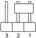
Set the 4-20 mA configuration by placing the jumper of connectors J14 (referring to B5) and J15 (referring to B6) as indicated in the figure on the left.
