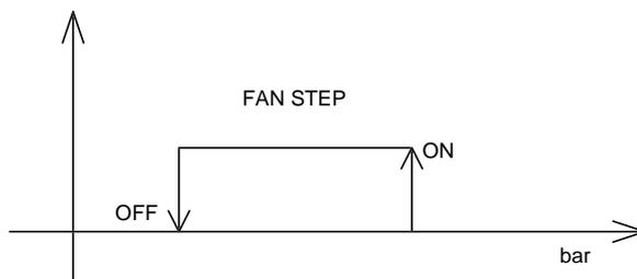
During the defrosting cycle the fans relative to the circuit undergoing such a procedure will be forced into the OFF status.
