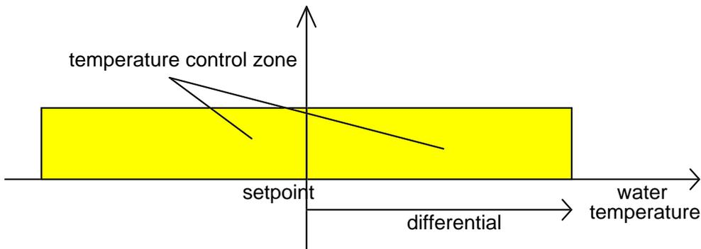
In the application shown in the figure above the set-point has been set so as to represent the **CENTRAL** point of the regulation zone.
