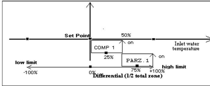
**Note:** the example above refers to cooling applications ('Summer' functioning mode). For heating applications ('Winter' functioning mode), the steps will be positioned specularly with respect to the set-point.
