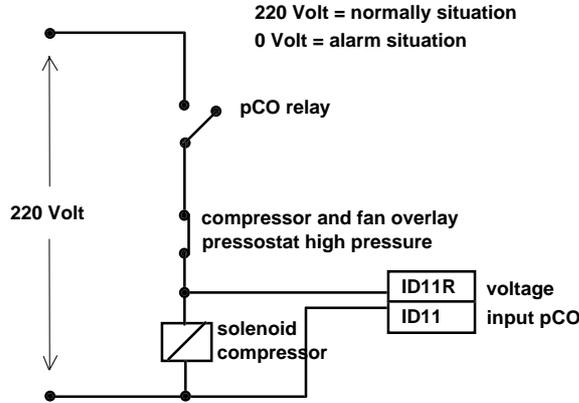
When pCO's relay enabling the compressor's functioning is closed and that relative to the high pressure pressostat is open, the 'high pressure alarm' will be detected through the 220 Volt input.
