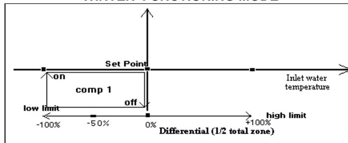
SINGLE COMPRESSOR UNIT WITH 1 CAPACITY-CONTROLLED STEP
